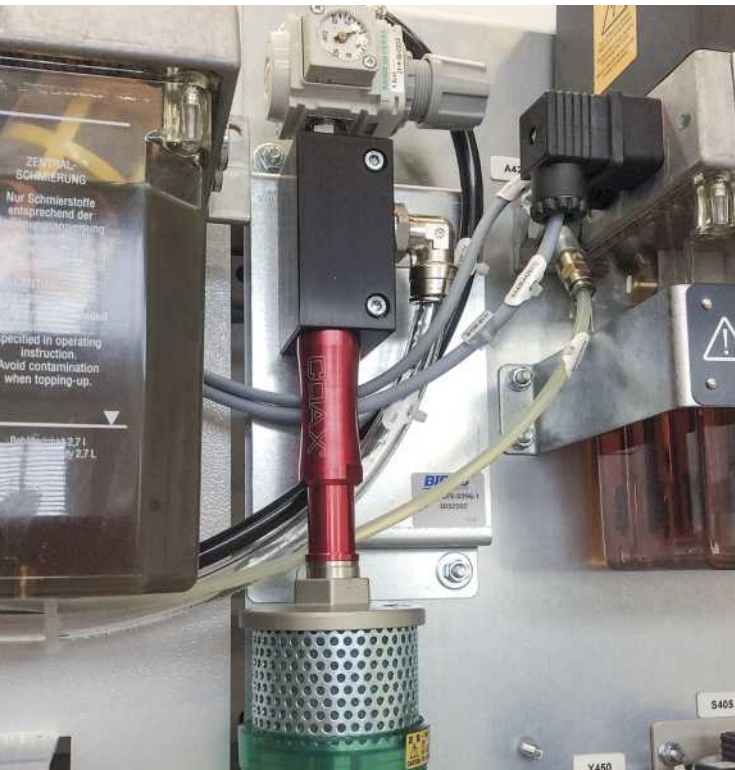
An optimized jet for extracting the oil-air mixture in the tool spindle uses around 57% less compressed air than before
